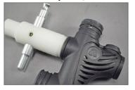
**POST ASSEMBLY TESTING:** Verify that the first stage regulator which the Powerline inflator will be used with has been recently serviced and adjusted to a stable MP of 130-145 psi (9-10 bar). Attach the first stage to a cylinder filled to 3000 psi (206 bar). Connect the Powerline inflator to the first stage via the quick disconnect MP hose. Slowly open the valve of the supply cylinder to pressurize the regulator.
