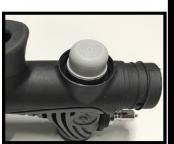
**5.** Fit the inflator bezel (p/n 15746) over the button cover (p/n 15100) and press down while rotating the bezel counter-
