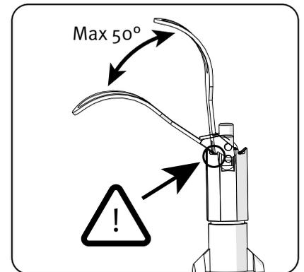
19. Reassemble the exhalation unit and the nut.
