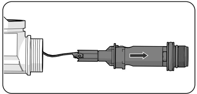
3. Remove the retaining ring and then pull out the valve insert from the connection nipple.
