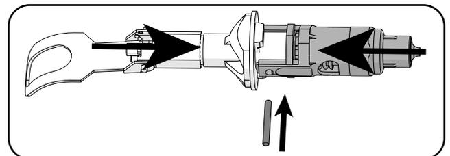
12. Assemble the valve insert sub assembly in the connection nipple and lock it with the retaining ring. Make sure to fit the retaining ring correctly.
