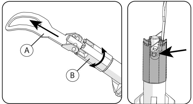
**IMPORTANT!** Never angle the lever more than 50 degrees as this may damage the contact surfaces on the lever support. When the valve insert is mounted in the breathing valve housing, the lever is prevented from angling more than 50 degrees. When the valve insert is removed from the breathing valve housing, the lever can be angled more than 50 degrees and thus damage the lever support.
