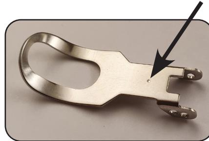
3. Check the lever height. If it is too low, replacement must be done before the next use, as this may be a sign of wear without visible damage.
