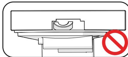
*Without lever bar:* Remove the exhalation unit except the locking ring. Push the locking ring upwards so that it lies against the edge. Check that you can see a gap between the lever and the upper edge of the locking ring. This test method is only for checking if the lever is too low and has no upper limit.
