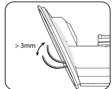
17. Use the lever bar to make sure that the lever is in the correct height. The lever must be in the upper area of the lever bar.
