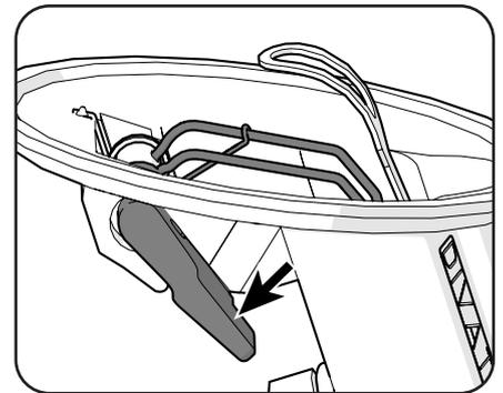
16. Make sure that the lever has a resistless movement of at least 3 mm.
