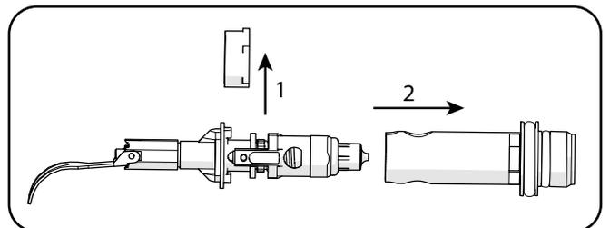
4. Press together the valve insert by hand so that the pin can fall out.
