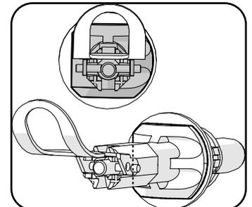
11. Assemble the valve insert with the new lever and lever support. Press the valve insert together and put the pin back.
